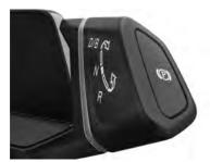
Fig. 114 On the driving mode selector: (2) button for the electronic parking brake.
