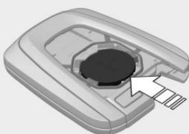
4. Insert a type CR 2032 battery with the positive side facing up.
