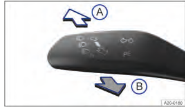
Fig. 87 On the left-hand side of the steering column: turn signal and main beam lever.
