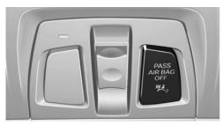
The indicator light for the front-seat passenger airbags indicates the operating state of the frontseat passenger airbags.
