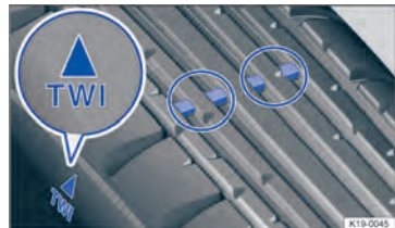
Fig. 185 Tyre tread: tread wear indicators.
