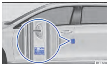
Fig. 184 On the driver door pillar: tyre pressure sticker (alternatively on the inside of the charging socket flap).
