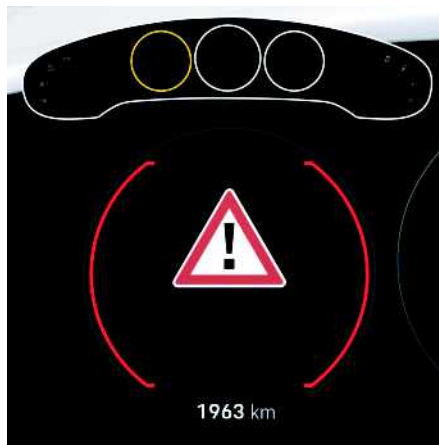
Fig. 219: Collision warning on the instrument cluster
